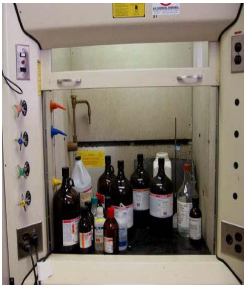
Improper Hood Usage
